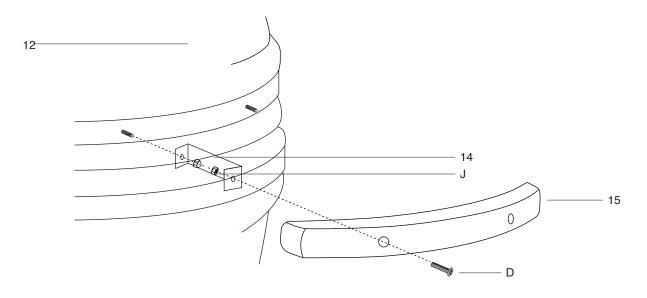
STEP 10 - To attach the handle (15) to the lid of the Kamado Grill (12) start by attaching 2x handle brackets (14) using the 2x pre-attached bolts and dome headed nuts. Attach the handle (15) to the brackets (14) using 2x bolts (D) and nuts (J).
