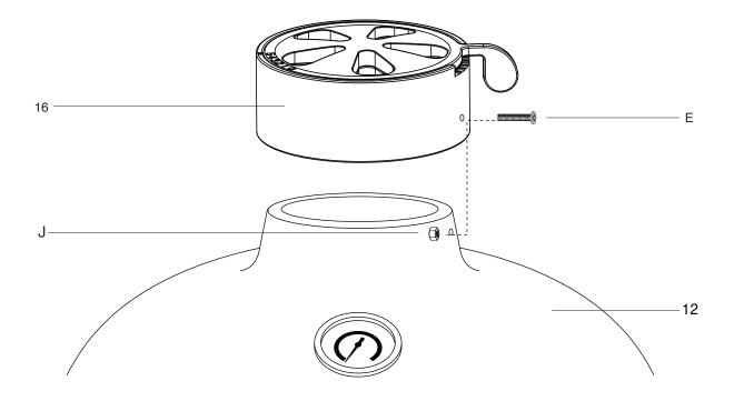
STEP 11 - To attach the top vent (16) to the Kamado Grill (12) place it on top and align both the bolt holes. Secure using 2x bolts (E) and nuts (J). Ensure that the top vent bolt is on the left hand side when assembling it.
